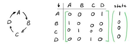
When the state [1, 0, 0, 0] — corresponding to state A — is fed through the system, we **multiply the vector through the matrix** and get [0, 1, 0, 0] — state B.
